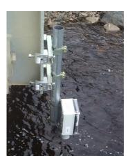
The small size and weight of the iGage makes deploying a new iGage very straight forward process. On the left is a typical bridge deployment using commercial off the shelf parts commonly available at retail and wholesale providers.
